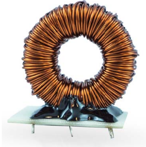
Figure 5. Traditional inductor using SiFe 40μ – 34μH @ 30Apeak
