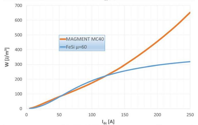
Figure 6:  $L=55 \mu H$ ,  $I=60A$  inductor corresponding to design case (c), same effective volume for a MAGMENT MC40 and a FeSi powder core toroid with  $\mu=60$ :
